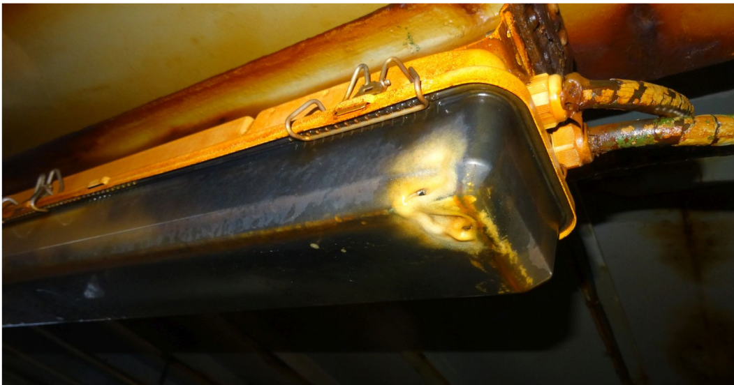
Picture 7 - ...which was fortunately killed immediately by water inside the light case
