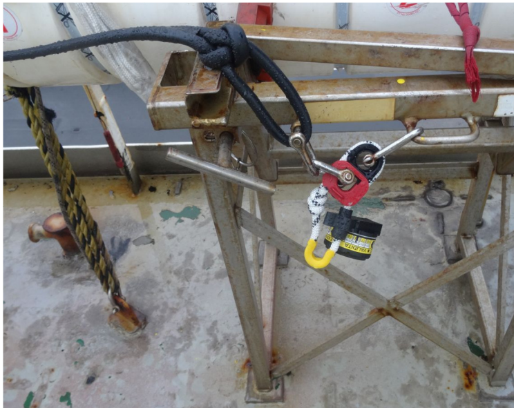
Picture 4 - not connected hydrostatic release unit
