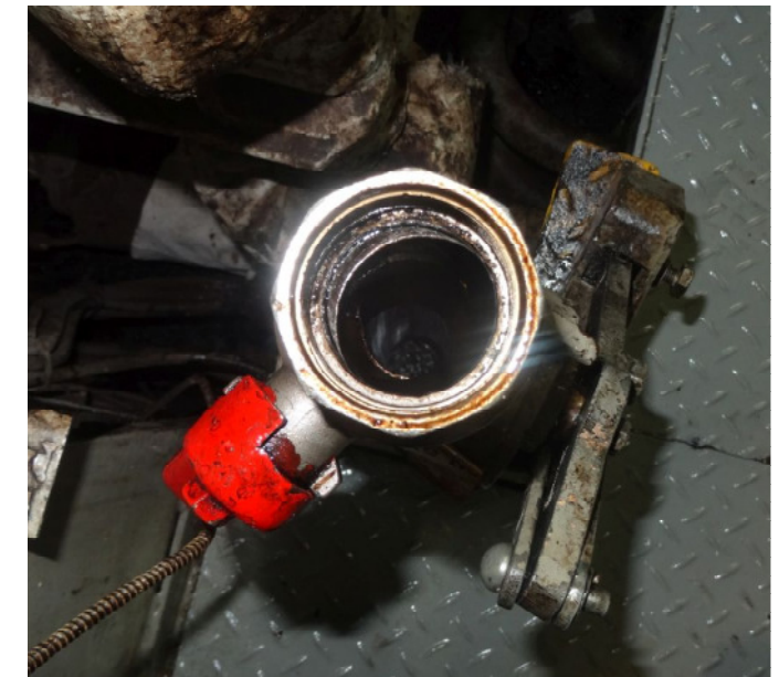
Picture 28 - damaged self-closing valve
