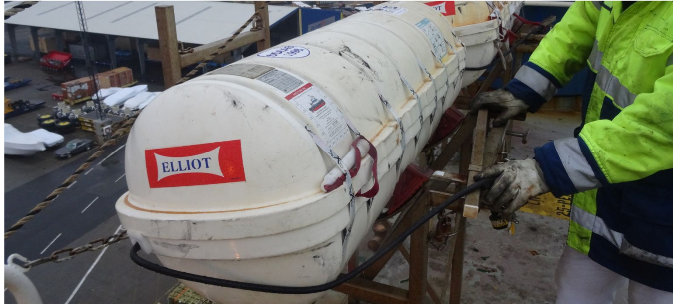
Picture 3 - liferafts only stored on board by painter line on weak link
