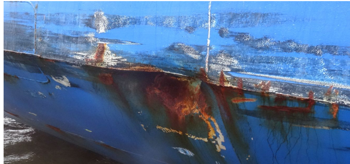
Picture 1 - bents on the outside hull, aft part
